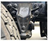
TORQUE ROD, SMALL EYE TR62-417M1
