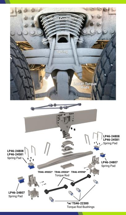
This walking beam suspension is similar in design to the Hendrickson HN suspension. It features bar pin end bushings but there are no center bushings for the beams to pivot on. Like the HN, the traditional center bushing is replaced by four narrow bolster springs (eight per vehicle.) The center of gravity has been lowered by designing the narrow bolster to straddle the beam in pairs compared to the HN where large single bolsters are mounted atop the walking beam.
