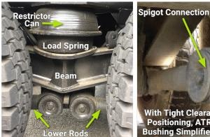
With Tight Clearance & Dowel Positioning, ATRO's 2-Piece **Bushing Simplifies Installation**
