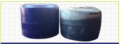
Load Springs subject to chemical attacks and should be replaced when worn. Otherwise ride height will be affected, causing numerous issues.
