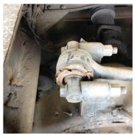
**Bushing Material Is Torn Or Cracked**
