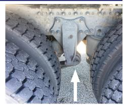
The UB20500-OS, an over-sized version (+.060"), is available if the rubber bushing has opened up the spring eye slightly. The spring must still meet specifications. If not, the spring must be replaced, not rebushed.
