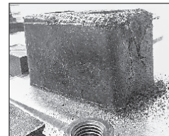
The OEM rubber bumper failed at 16,250 cycles.
