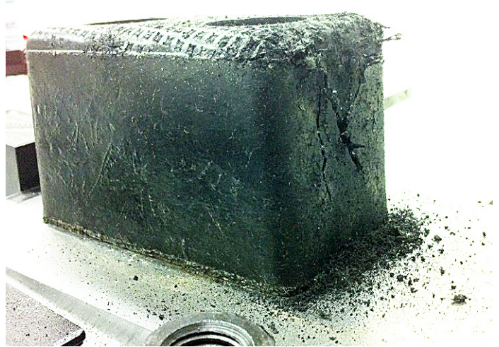
OEM Rubber Bumper at 16,520 cycles
