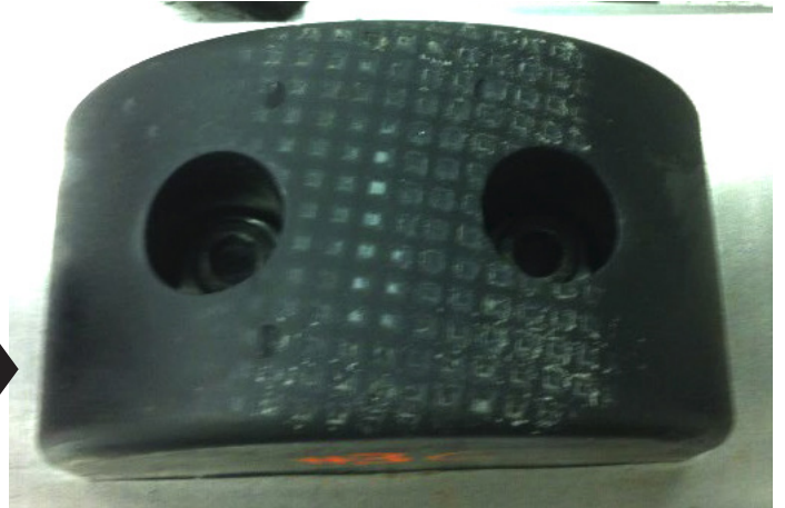
ATRO Polyurethane Bumper at 250,000 cycles
