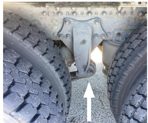
The **UB20500-OS**, an over-sized version (+.060"), is available if the rubber bushing has opened up the spring eye slightly. The spring must still meet specifications. If not, the spring must be replaced, not rebushed.
