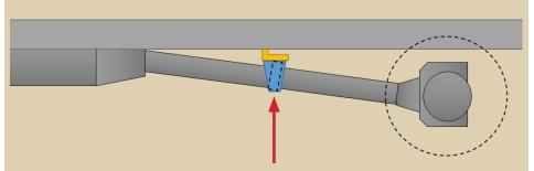
With the ATRO self-aligning carrier bearing assembly, there is no need to shim because the center is allowed to pivot + or - 10 degrees.\*
