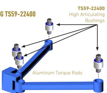
rapidly wear the torque rod bushing. In severe cases, it can contribute to breaking the aluminum torque rod. ATRO designed a torque rod bushing with a higher allowable side to side, conical movement in the bushing. This bushing uses an oval pin configuration and articulation voids designed into the polyurethane. This design allows the bushing to move 12° in both directions, 24° total movement. This greatly extends the bushing life and relieves the stress on the torque rod.
