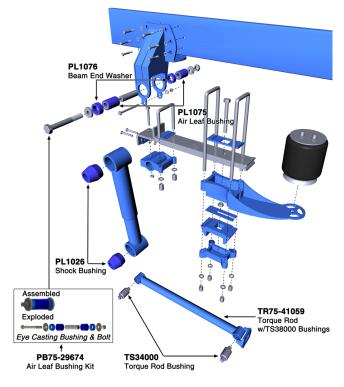
This air suspension has a maximum capacity rating of 40,000 pounds. This suspension, like the Low Mount Air Leaf, does not have lower radius rods like those found on the Air Trac. The air bags are supported on a paddle.
