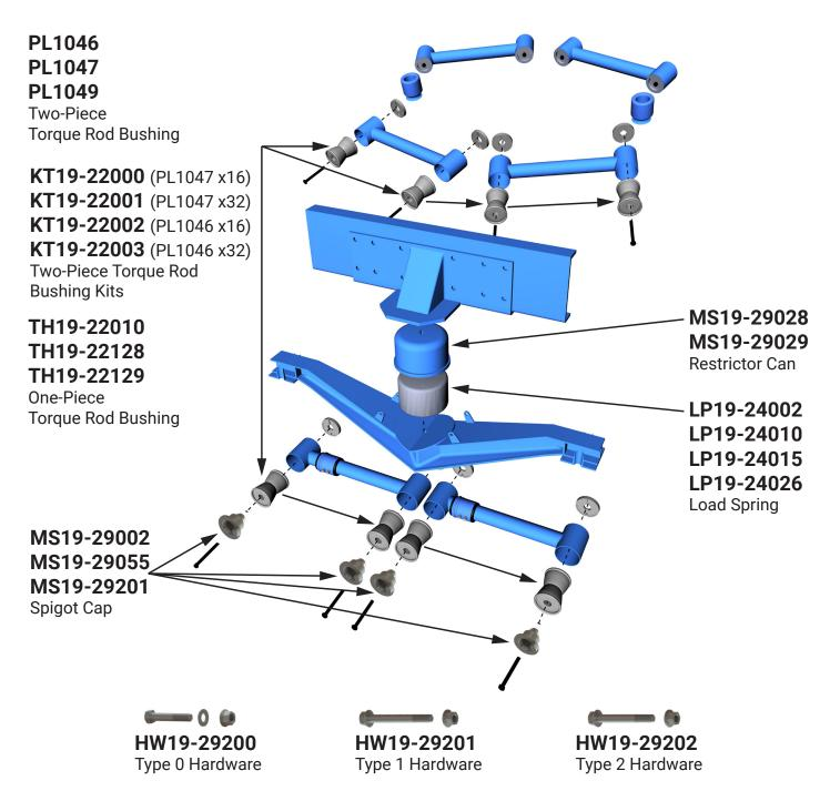
\*ATRO's two-piece bushings allow for easier installation by eliminating the interference between the spigot and ID. Simply slide one half of the two-piece bushing over opposite spigot ends and install the bare rod, install the second half of the bushings, caps and bolts. Reduces install time by 30% to 50%.
